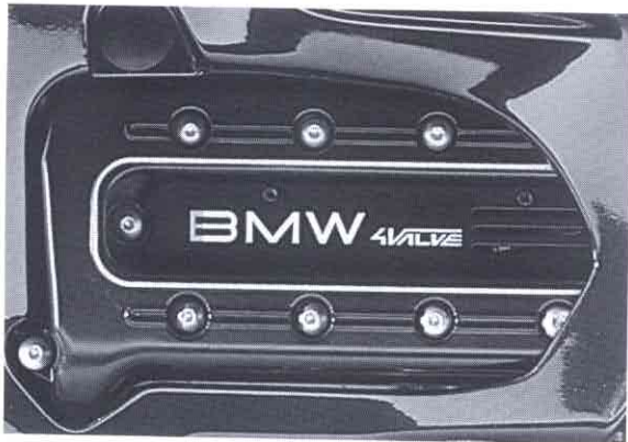
The valve cover characterizes the looks of the four-cylinder 16-valve powerplant.
