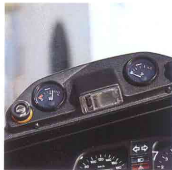
5 Keeping exact time in a new age. The BMW digital clock powered by the on-board electrical system is now also available on our GS machines (from '91 model on).
