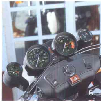
6 The BMW voltmeter shows you the exact battery charge, and the quartz clock (Boxer) or digital clock (K-Series) tell you the exact time.
