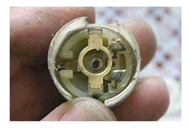
Here is the bottom part of the old switch. The contacts here are definitely in bad shape. These could be cleaned up but I replaced mine.
