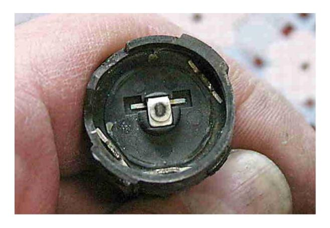
Here is the inside of the new housing with the switch contacts. Clean out this area until it looks like this.
