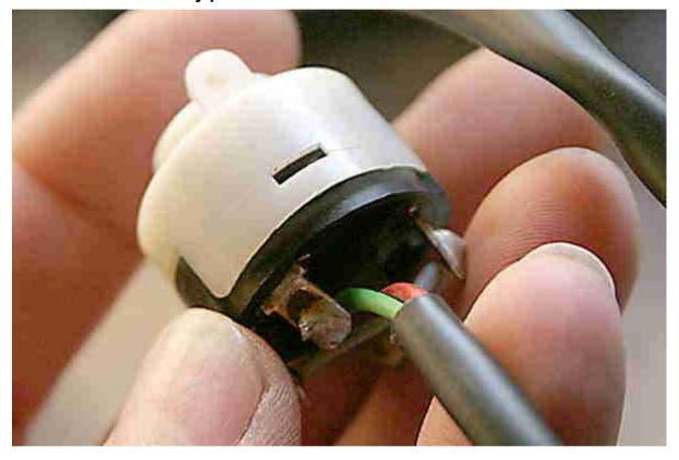
Hold this side down when you separate the halves. Notice that the Y shaped contact has two tabs that fit in slots. The straight contact has a small tab on each end which also fit in small slots. This is my new switch.
