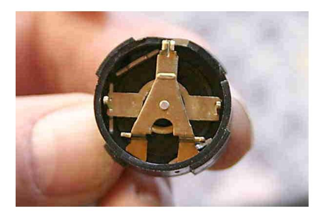
This photo shows the ON position. Notice that the straight arm connects the two switch contacts on the left and the right side here, and the Y arm connects the centre and bottom left. The arms never contact each other.
