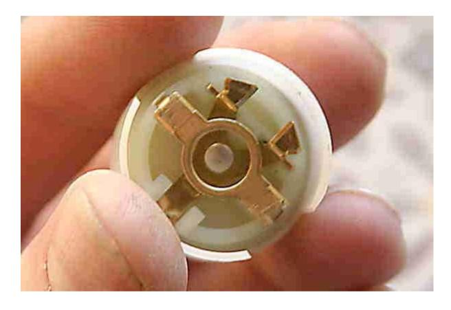
Make sure the switch is in either Park or ON position before pushing the black housing down into the white housing.
