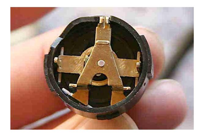
Before reassembly, put the moving contacts in their positions as shown here below. Make sure the 4 small springs below are in place first.
