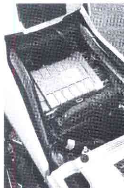
Bosch Digital Motor Electronics (DME/Motronic) control box resides under seat on top of battery, ABS black box directly in back of battery.
