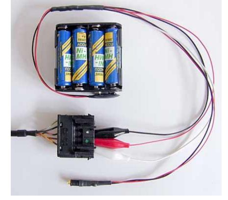
Any good sensor should light the LED until something metallic, like a feeler gauge, is introduced in to the sensors gap, the LED will then go out.
