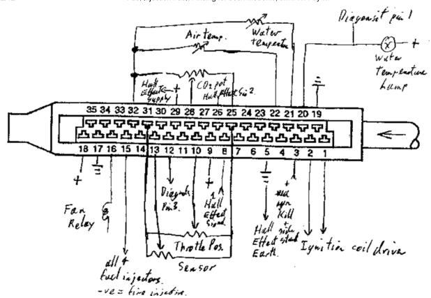
All the connector numbers refer to the motronic connector above, unless specified other wise. This is done so that there is a common test connector following wires and connectors. This makes the test simple. If a test fails then you should test the interconnecting wires and connectors. It may the procedure here does not check for shorts to the chassis, you should do these while flexing any and all wires from this connector to the item
