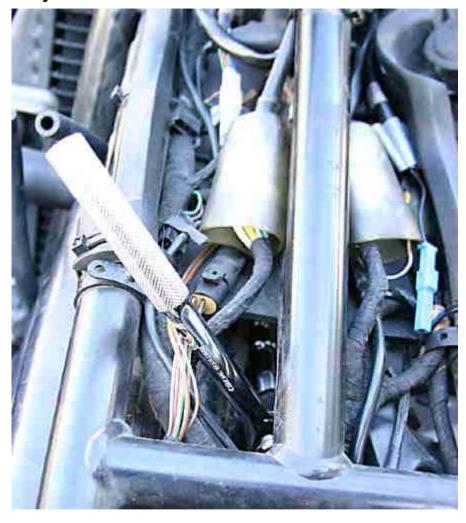
And here is the view with the airbox removed. Once the clamp above is loosened, the aircleaner is easy to slide out. First, unclip the three clips holding the airbox halves together. Then slide the filter out carefully. then the top of the airbox should come out. There is a wire attached to it that you should leave alone. Just move the top to the side as much as possible, there is no need to actually move it
