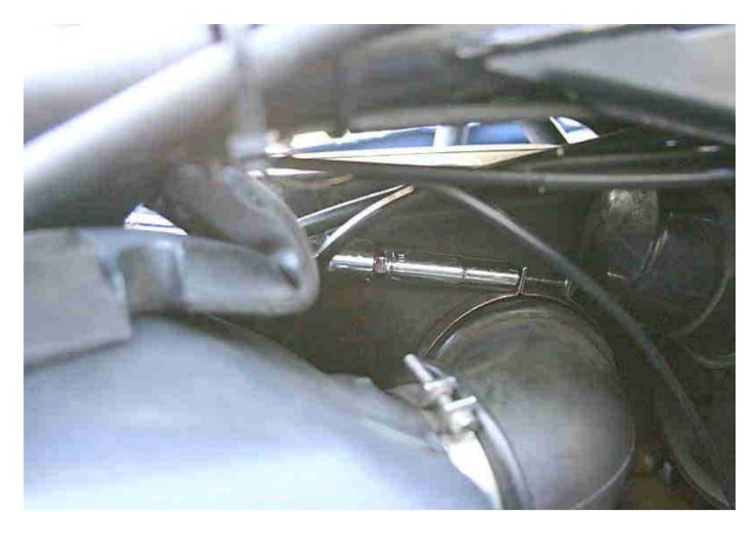
Here is a view from above of how the ratchet is positioned to remove the hoseclamp. It is a painfully slow process unscrewing the clamp, as the ratchet can
