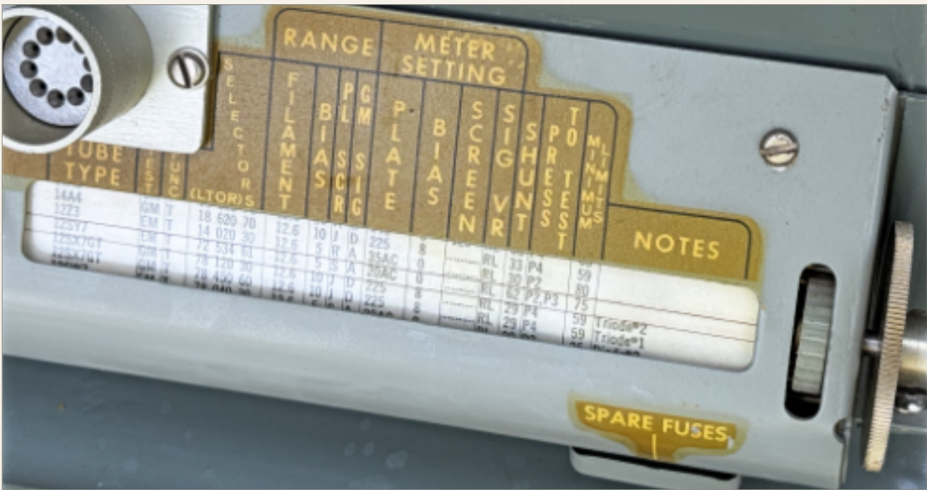
Above: The Tube Test Data Roll Chart – The TV-2/U carries its tube-test data on a roll chart mounted inside the cover. The chart is divided into two sections, with tube types arranged in ascending numerical and alphabetical order. Repeated headings identify the tube type, the sequence in which the tester controls must be set, and the minimum acceptable percentage of rated transconductance to be read on the PERCENT QUALITY meter. For each listed tube, all required switch and control settings appear directly beneath these headings.
