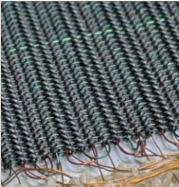
Detail of the core memory in the “real” PDP-8. Each core is less than one millimeter across.
