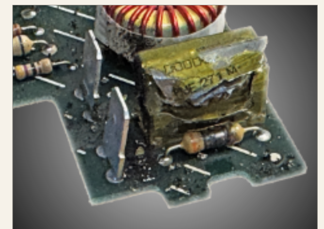
Photo: The exploded RIFA capacitor described in the text. Note that its failure also caused the 30 \Omega resistor R882 to burn. This is a useful reminder of what the “safety” rating of an X2 capacitor actually means: it does not guarantee that its failure cannot damage other components. If the surrounding circuitry is not adequately protected, a failing capacitor may still create potentially hazardous conditions.
