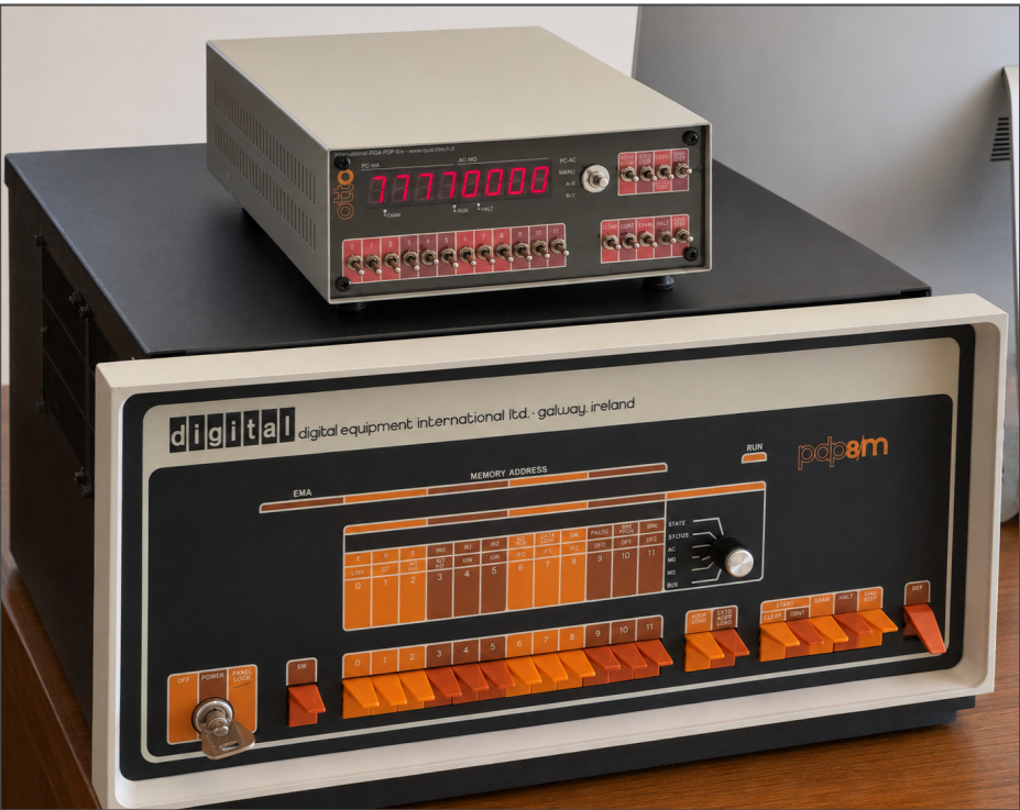
OTTO compared with the “real” PDP-8, built in Europe, as proudly stated by the inscription on the front panel. Note the key-operated power switch: a real security key. Evidently, not everyone was allowed to turn on a real computer...
